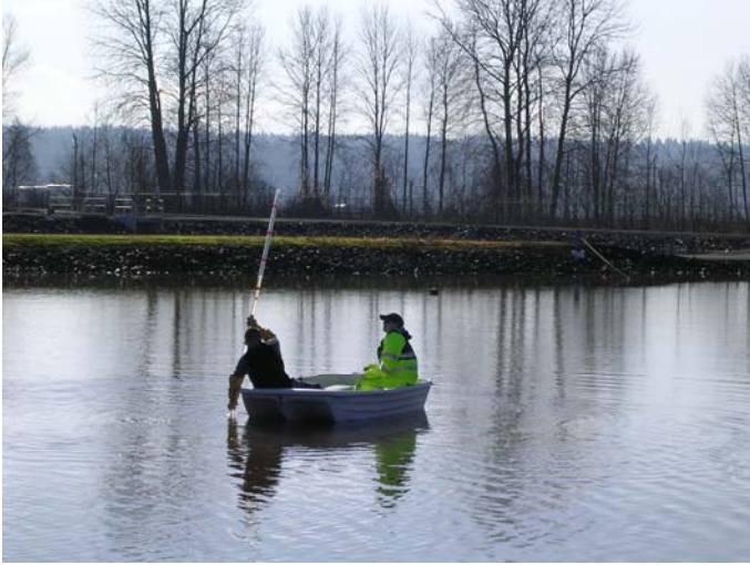
Measuring sludge depth in wastewater lagoon
